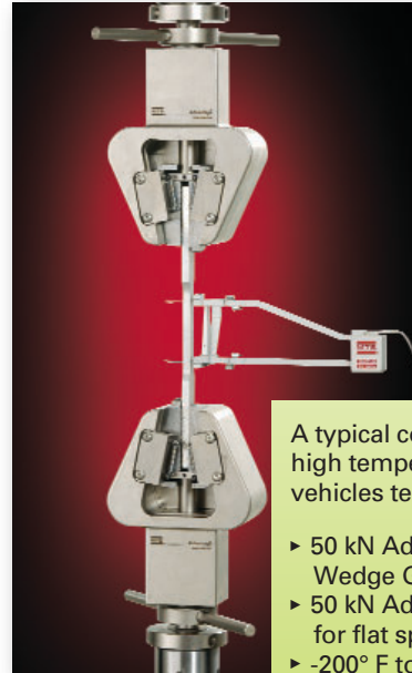
(shown with 634.25 extensometer)
